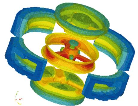
*Figure 1: Expanded view of a cast wheel with mold and core presenting the temperature distribution. Simulation realized with ProCAST.*
